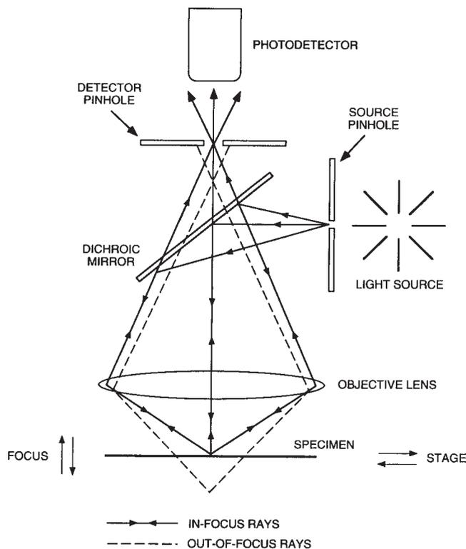
Fig. 2. The light path in a typical LSCM is based upon that of a conventional reflected-light wide-field epifluorescence microscope, but with pinholes placed in front of the light source (the point source is now a laser) and in front of the photodetector. The pinhole at the light source, the focused point in the specimen, and the pinhole in front of the detector are all confocal with one another.
