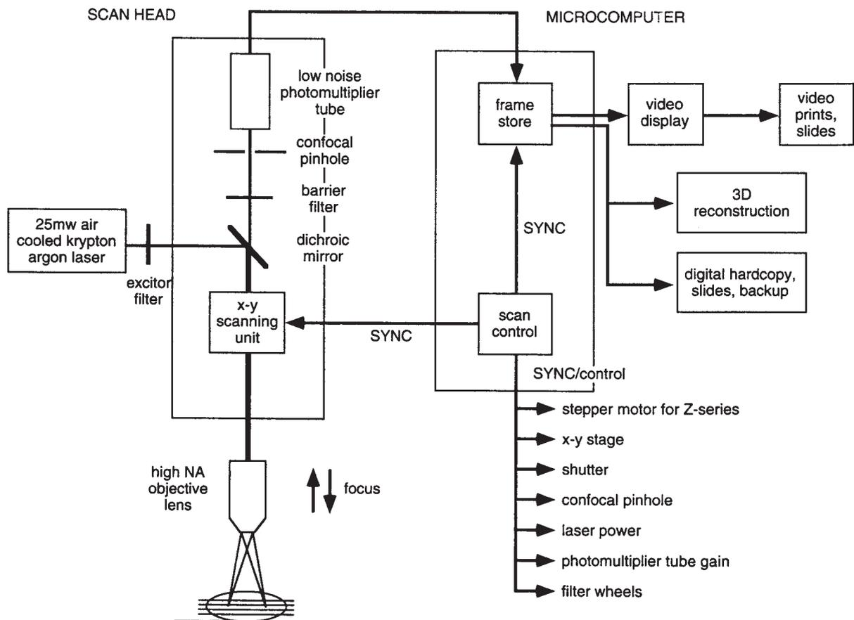
Fig. 3. Information flow in a laser scanning confocal imaging system.
